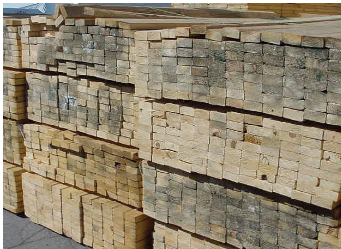
Example of green & black mold caused by wood getting wet in transit.
