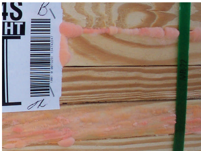
Another example of pink mold caused by improper kiln drying.
